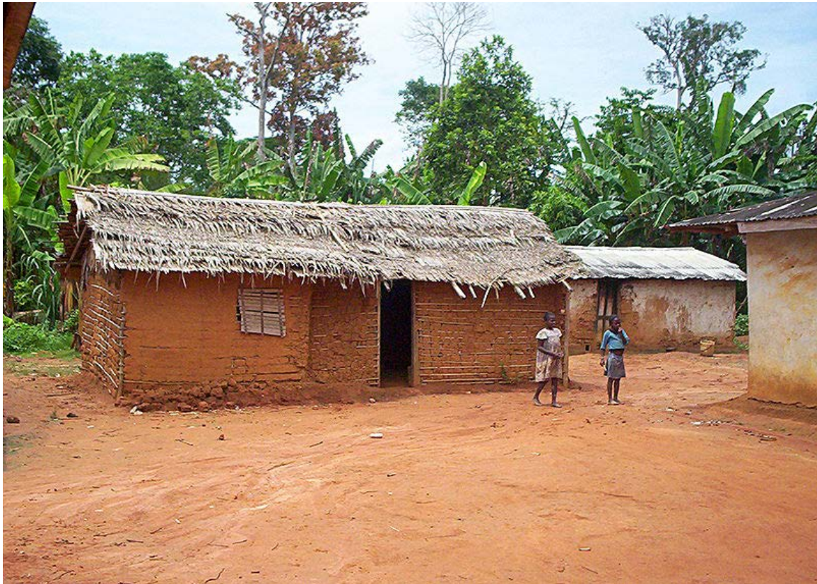
Cameroon, a wattle and daub house, roofed with banana leaves
