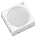
Figure 9: LED package – First sample and package dimensions [1]
