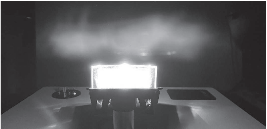
Figure 6: Light distribution of the demonstration device. Although illuminated with white LEDs the VCA image is green, caused by the wavelength selectivity of the hologram.
