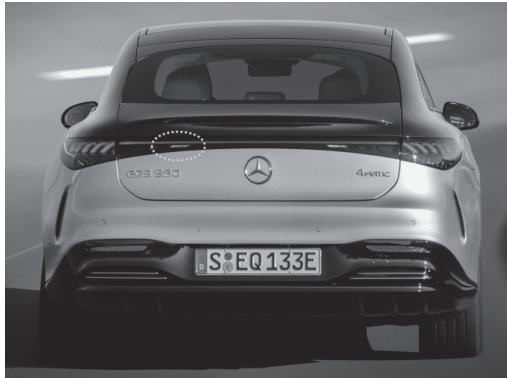
Figure 1: Appearance of the rear lamps with clear functional fields for the reversing light on the vehicle [4]
