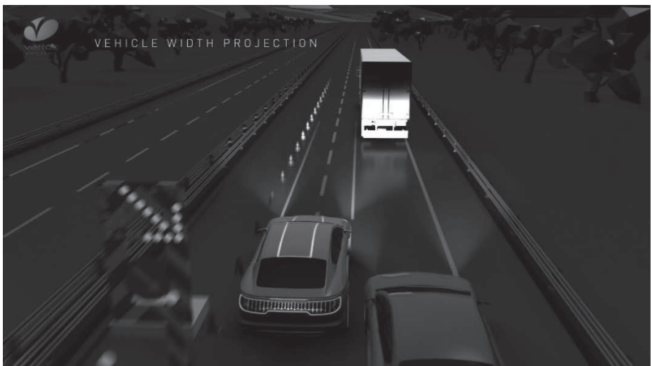
Fig. 2 : Guiding lines in construction zone areas
