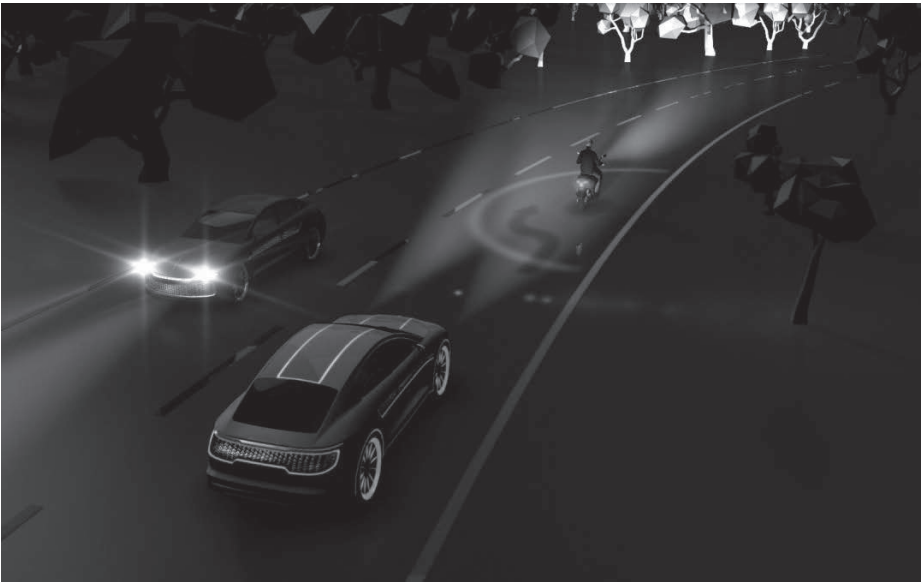
Fig. 3 : Safety distance recommendation when overtaking
