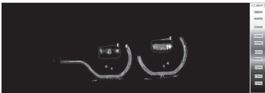
Figure 2: Luminance picture of future Laser-headlamp
