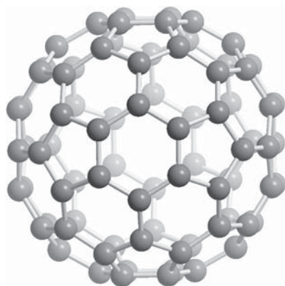
Figure 1.11 Icosahedral C_{80} cage of \text{Sc}_3\text{N}@C_{80} .
