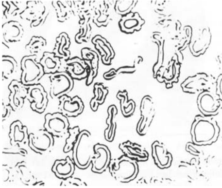
Fig. 1-14 Cross-sections of hollow fibres
