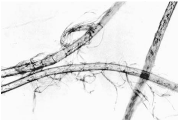
Fig. 1-11 Wet fibrillated polynosic fibres (lyocell fibres have similar properties)
