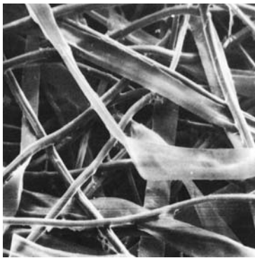
Fig. 1-15 Bonding of nonwoven bonded fabrics with hollow fibres
