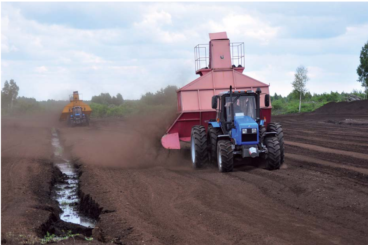
Photo 14: Industrial milled peat extraction in Tsna, Minsk oblast (Belarus, H. Joosten, June 2014).
