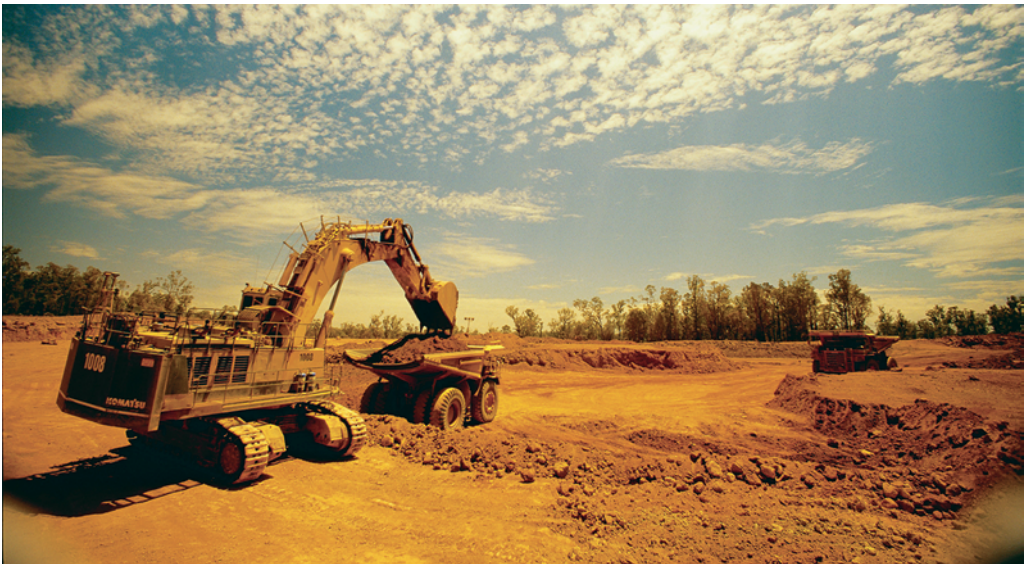
Fig. 1.1 (Plate 1.1). Bauxite extraction at Huntley mine, southwestern Australia. On the Darling Plateau, bauxite is part of a mature soil profile developed over Archean gneiss and granite. The area is covered by woodland (the jarrah, or Eucalyptus marginata forest). Mining depends on the availability of land. Its social acceptance requires rapid re-establishment of the native ecosystem. Reproduced by permission of Alcoa Inc.
