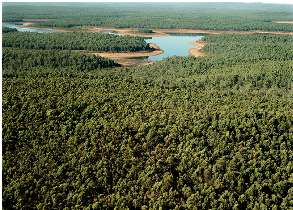
Fig. 1.2 (Plate 1.2). Rehabilitated jarrah forest covers former extraction panels of Huntley bauxite mine in front of the lake. Part of the remarkable success is due to skilful use of the natural soil seed bank. Reproduced by permission of Alcoa Inc.
