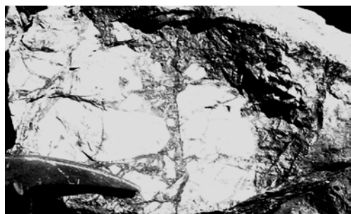
Fig. 1.39. Breccia ore at Mammoth copper mine near Mt. Isa, Queensland. Supergene secondary chalcocite (grey near hammer) replaces primary chalcocite and pyrite in veinlets within quartzite (white).
