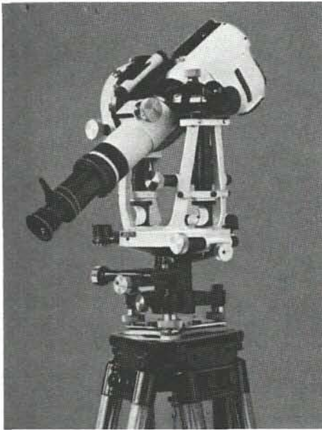
Figure 26 First Boßhardt-Zeiss reduction tacheometer
