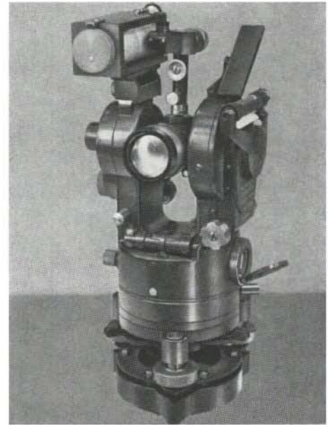
Figure 15 Ewing distance- and height meter attached to Watts theodolite
