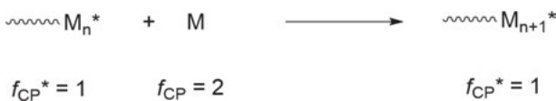
Scheme 1.3: Number of functionalities of a growing active polymer chain ( f_{CP}^* ) and corresponding monomer.
