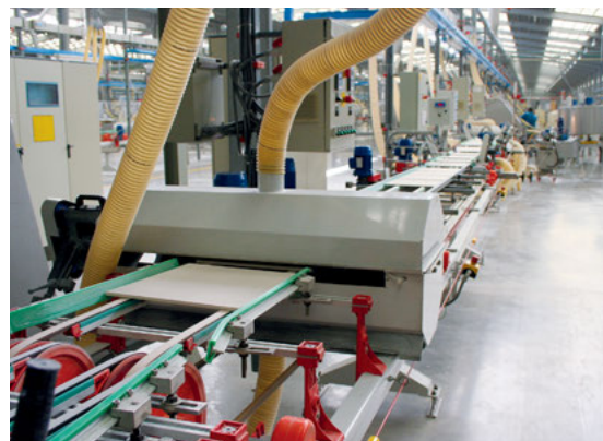
Highly automated mass-production of dry-pressed floor tiles at Porcelanosa, Castellón, Spain. Industrial production settings such as these can output several thousand tiles per hour.
