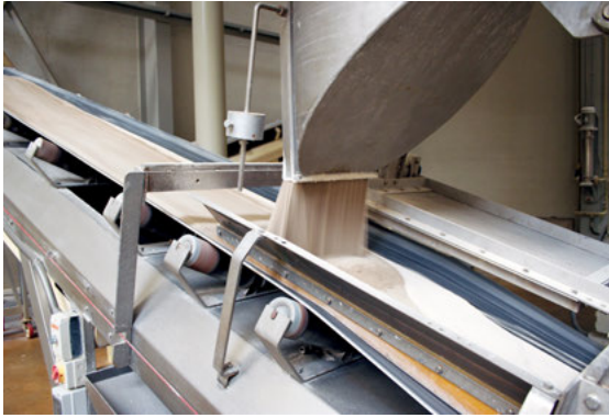
Automated clay body preparation in a high-volume production system.
