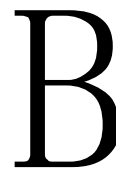
Fig.6 one machining region consisting of one outer contour and two inner contour
