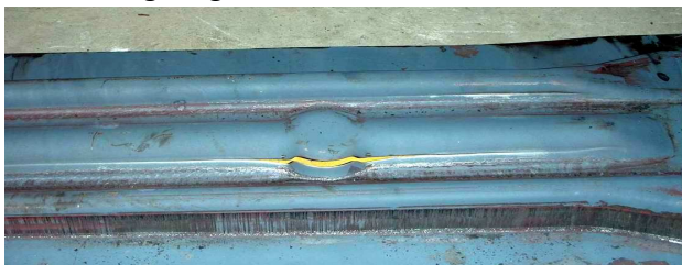
Figure 8 Experiment result of hot-stamping of collision beam
