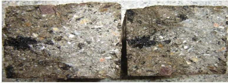
Figure 1 Cold-recycled mixture mesoscopic structure
