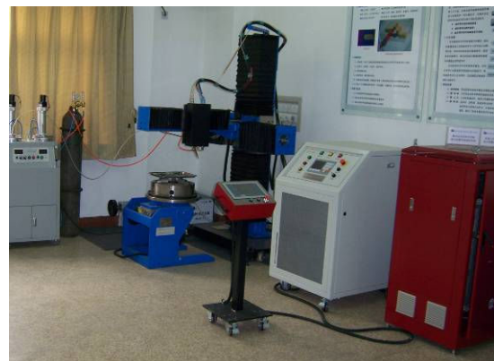
Fig.10 The high power diode laser system with manipulator operating
