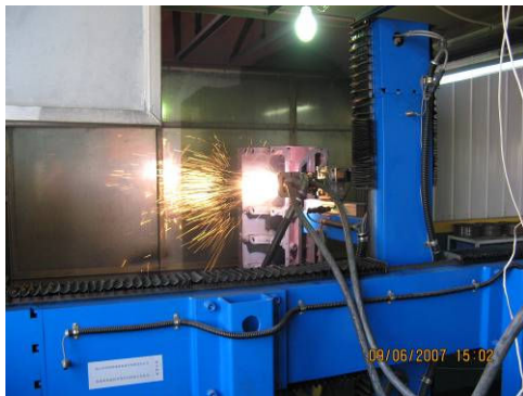
Fig.4 Process which the AHVAS technology remanufactures a discarded STYER engine block
