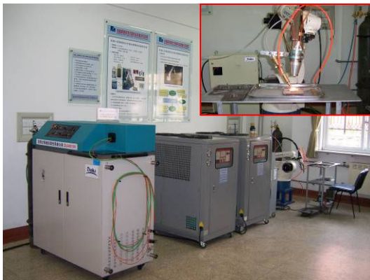
Fig.9 Fiber coupled solid laser system with robot operating
