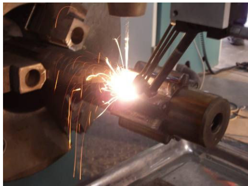
Fig.8 Automatic laser cladding remanufacturing to the tooth surface of heavy load gear
