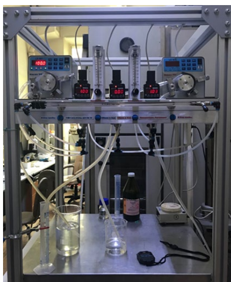
Figure 3. Installation for measuring water permeability and retention capacity.
