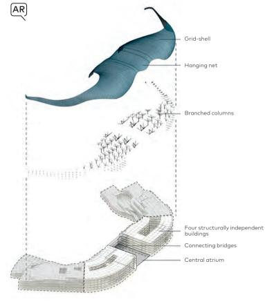
distortion. Furthermore, eliminating diagonal members makes the net more transparent, reduces the number of rods and panels, and significantly simplifies the nodes.
