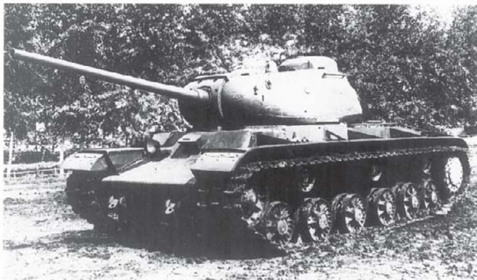
The final production variant of the KV series was the KV-85. This was a stop-gap improvisation, mating the new turret from the IS-85 tank with a modified KV-1S chassis. The new IS-85 turret had a wider turret ring than the KV-1S, so a fillet had to be added to the hull sides to provide the added space.
