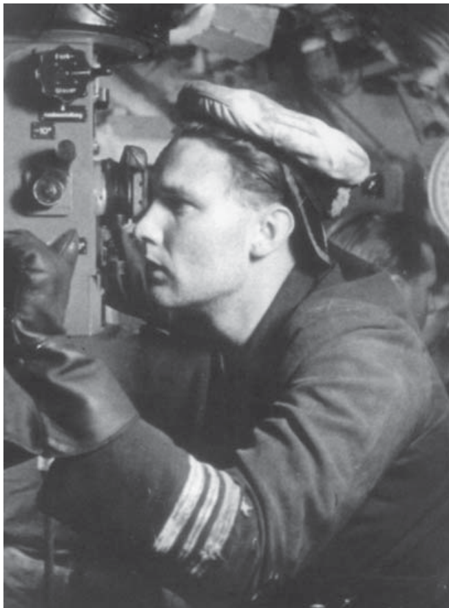
Kapitänleutnant Kurt Diggins, commanding the Type VIIC boat U-458, is shown at the navigation or 'sky' periscope in the relatively spacious control room. This larger of the two periscopes was used predominantly for scanning the horizon and sky for enemy ships and aircraft, and also to take bearings. KL Diggins survived the sinking of his boat in August 1943, and outlived the war. (Deutsches U-Boot Museum)
