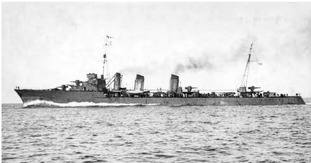
Left: Tigre running trials on 14 October 1925. She was the fastest of the class, achieving an impressive 36.7 knots with 57,200CV, which was widely reported and had a considerable impact abroad. (US Navy NH 88960, courtesy of A D Baker III)
