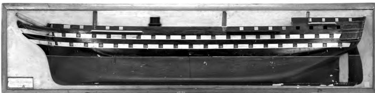
Official half-model of Duncan , the final development of Edye’s brilliant design of Agamemnon and the only one of the class completed as an unarmoured ship. (© National Maritime Museum L0818)
