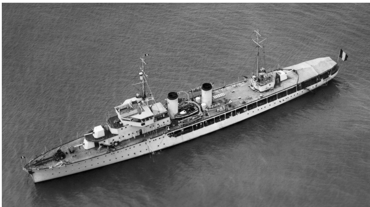
An aerial view of the nameship of the class, Bougainville (A1), at Majunga on the northwest coast of Madagascar, during her first deployment to the Indian Ocean. She has yet to be embark a reconnaissance aircraft or the planned minesweeping paravanes amidships, so the after part of the shelter deck is unusually uncluttered. Note the wooden planking on the forecastle and shelter decks, and the canvas awnings over the quarterdeck and the bridge decks. (Forces Aériennes Françaises de Madagascar, courtesy of Jean Moulin)
