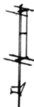
Type 279 (both masts) Type 279M (one mast only, first model introduced Jan 1940, virtually same as Type 79)
