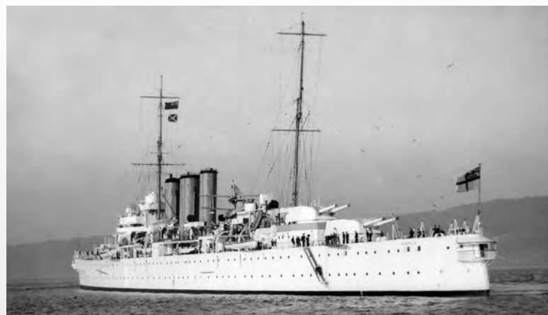
Above: HMS Norfolk , a later 'County' class cruiser, emerged from a 1937 refit with twin 4in anti-aircraft guns, part of a rearmament package proposed by the 1932 Naval Anti-Aircraft Gunnery Committee. The single centreline anti-aircraft director (aft) with which the ship was completed was replaced by a pair of such directors abreast the bridge. Other improvements were a pair of octuple pompoms, the most powerful existing light anti-aircraft weapons, abeam the after superstructure, and a pair of the new quadruple 0.5in machine guns on platforms abeam the gap between the first and second funnels. The inter-war Royal Navy invested more in anti-aircraft firepower than any other, and was air-conscious to the point that additional deck armour for capital ships was justified as a defence against bombing. The 4in gun was particularly important because it was assumed that enemy bombers would attack from medium altitude, hence could be engaged at a considerable distance and their formations broken up. Unfortunately the Royal Navy opted too soon for a fire-control system which depended on the controlling officer's estimate of the speed of the approaching aircraft. Just before the Second World War the Director of Naval Ordnance wrote that this had been the wrong choice; he was about to test a tachymetric (speed-measuring) system (which, probably unknown to him, the US Navy already used). He expected the new system to enter service in 1941. The ship's DF array is just visible near the juncture between the foremast and its topmast, just below the crow's-nest.
