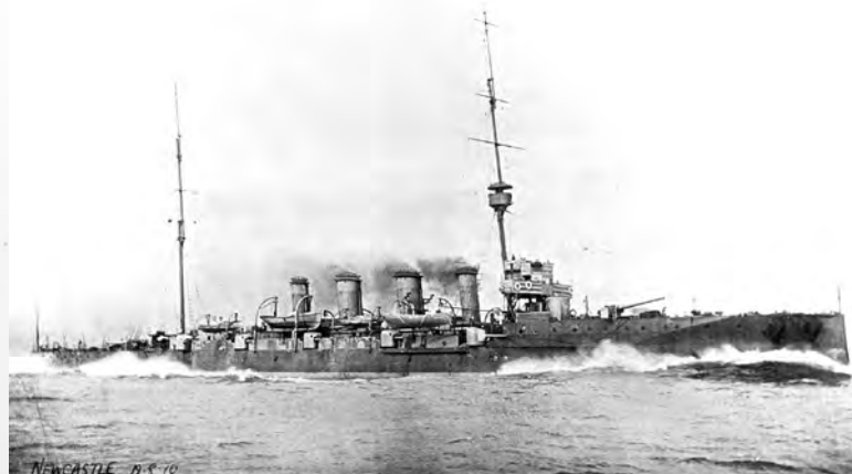
HMS Newcastle shows the effect of short funnels in this 19 August 1910 photograph.
