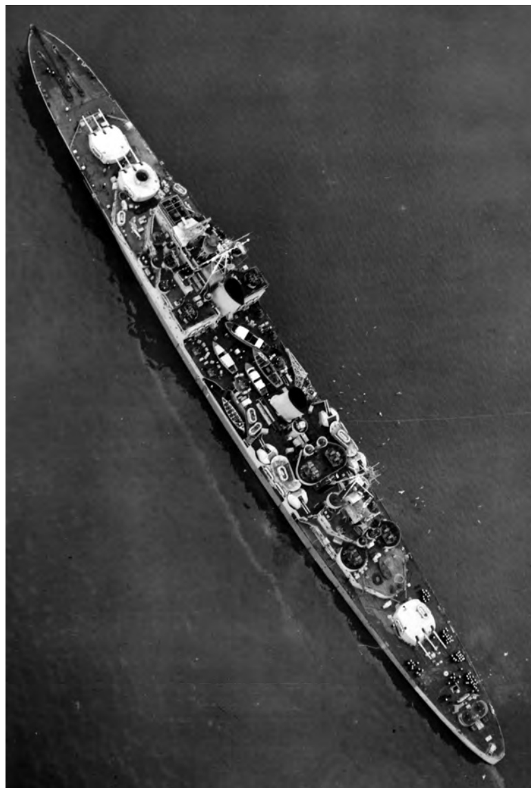
Above: By late 1943, drastic changes were needed to free topweight and space for further additions, particularly for more close-range weapons. HMS Birmingham is shown on 23 November 1944 at Hampton Roads after a refit in the United States (Norfolk Navy Yard, July 1944 – 28 November 1944), her 'X' turret having been removed. She retained the two quadruple pompoms atop her former hangar, but the refit added four quadruple Bofors aft plus five single and two twin Oerlikons. She already had two single Oerlikons (seven fitted during a Simonstown refit, 5 March 1942 – 1 April 1942, but five removed during the next refit) and eight twin Oerlikons (added during a Devonport refit, 23 April 1943 – 21 August 1943). Note the short depth-charge track right aft, a standard installation on board British cruisers from the First World War onwards.
