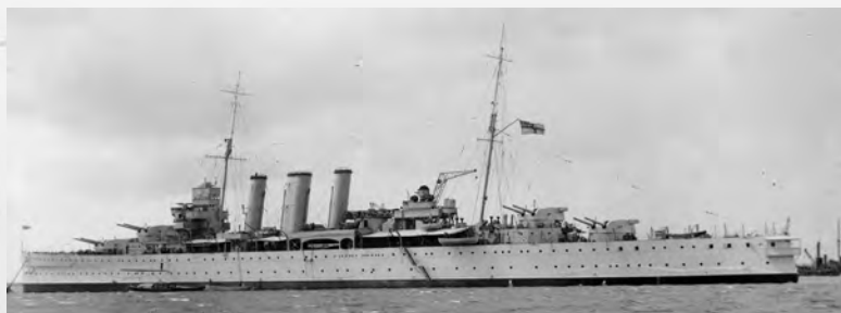
Above: HMS Kent emerged from a 1931 refit with a catapult, an important feature because an aircraft gave a cruiser a much better chance of detecting raiders. Within a few years the Royal Navy was intensely interested in the offensive potential of catapult aircraft, but the one shown here was limited to spotting duties. Aircraft were included in the design (the ships were completed with a foundation for a catapult) but initially were omitted to avoid exceeding the 10,000-ton Washington Treaty limit.
