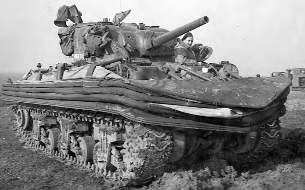
Sherman DD (duplex drive) tank with floatation skirt folded.
