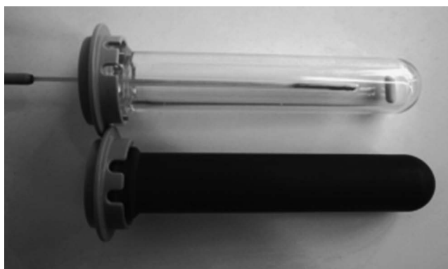
Figure 1.5 Reaction vial made from sintered SiC (lower). For comparison a standard 10 mL Pyrex vial with a snap cap, internal FO probe and a magnetic stirrer bar is also included (upper). Reproduced from B. Gutmann, Chem. Eur. J. , with permission from John Wiley and Son. Copyright © 2010 WILEY-VCH Verlag GmbH & Co. KgaA, Weinheim. 31
