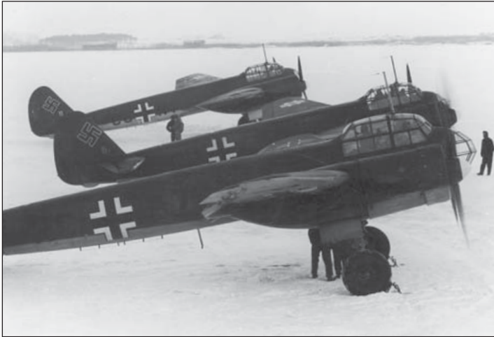
A trio of early Ju 88A-1s from a training unit. Note the high demarcation line between upper and lower camouflage surfaces of the furthestmost machine, and the small numerals on the tailfins. The snow on the ground would suggest that these are machines of Lehrgruppe 88 , photographed in the winter of 1939-40
