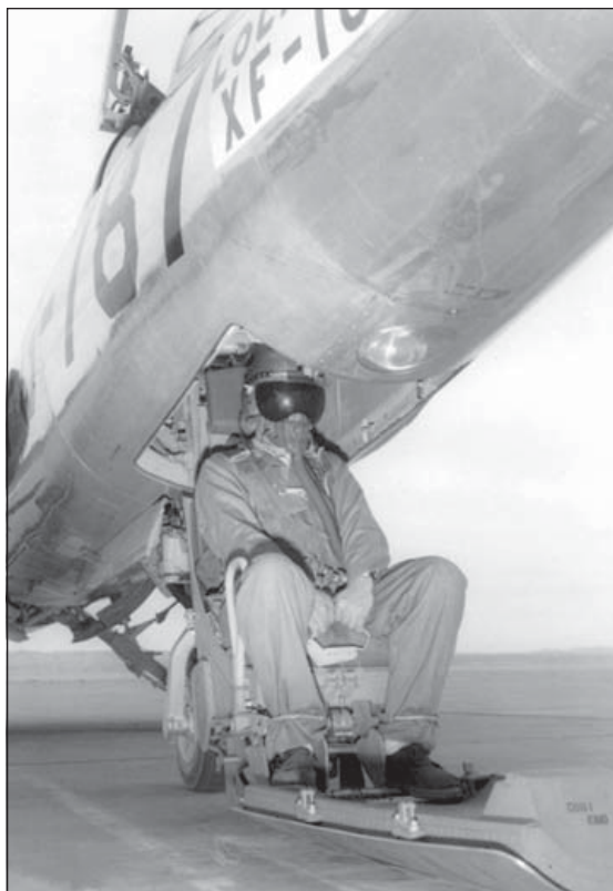
The original downward-firing Stanley B ejection seat, connected to an ejectable lower fuselage hatch, offered simplicity and light weight, but it presented problems at altitudes below 1500 ft, where the pilot was supposed to eject with the aircraft inverted – albeit with a greater risk of back injury due to negative-g. High-altitude ejections were, in any case, rare. Seen here with the second XF-104 (53-7787), the seat had an exit route that obviously left little room for error (Lockheed)
