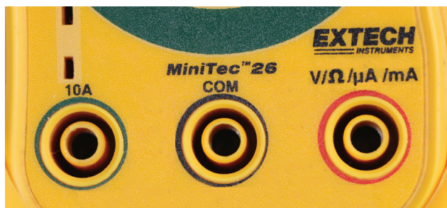
Figure 2-10. This meter allows you to measure volts, ohms, \mu\text{A} , and mA all from one socket.
