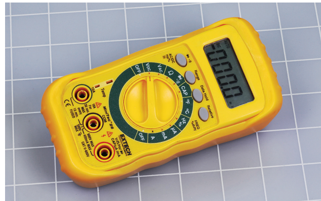
Figure 1-2. An auto-ranging meter.
