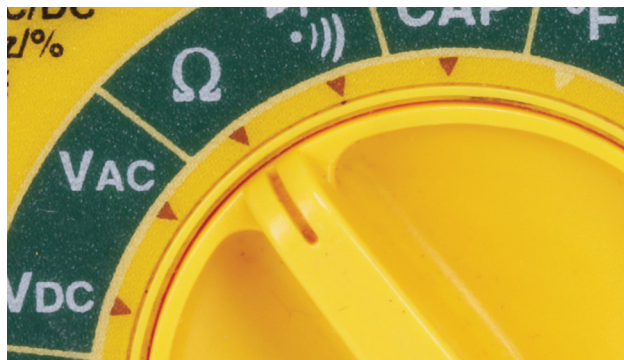
Figure 1-22. Selecting resistance in an auto-ranging meter.
