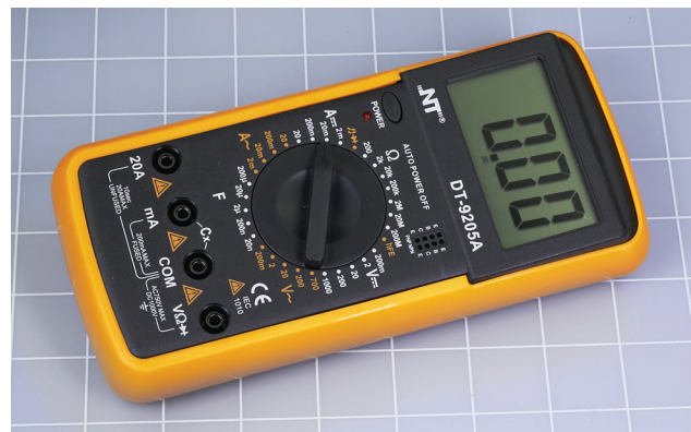
Figure 1-3. A manual-ranging meter.
