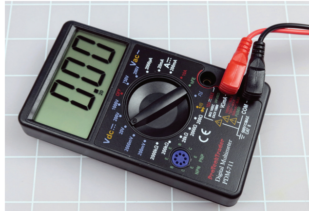
Figure 1-1. A bare-bones digital multimeter. The squares behind it are at intervals of 1 inch.
