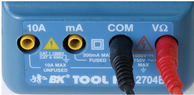
Figure 1-19. Where to plug in the meter leads.
