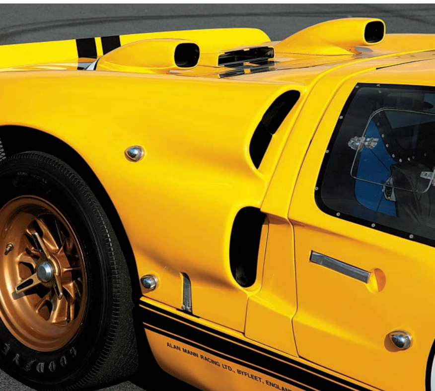
Copious vents were required in order to cool the GT40's huge 427-cubic-inch big-block V-8.
