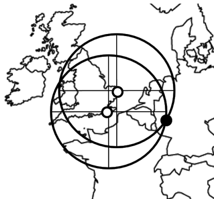
Figure 1.6 The Oboe system: the picture depicts two Oboe ground stations on the channel coast of England and the intersection of the two circular lines of position over western Germany, marking the target area.
