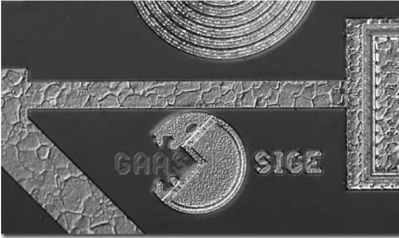
Figure 1.14 Headline News: "SiGe 'Pac-Man' gobbles up GaAs competition!" (Used with the permission of Michael W. Davidson, Florida State University.) This SiGe Pac-Man was found on a SiGe RFIC designed by TEMIC Semiconductors. Pac-Man was originally designed by Toru Iwantani and programmed by Hideyuki Mokajima and his associates. The name Pac-Man is derived from the Japanese slang "Paku-paku," which means "to eat." Originally, the Japanese named the game "Puckman," but it was changed to "Pac-Man" upon launching in the United States. Pac-Man is the best-selling video game in history.
