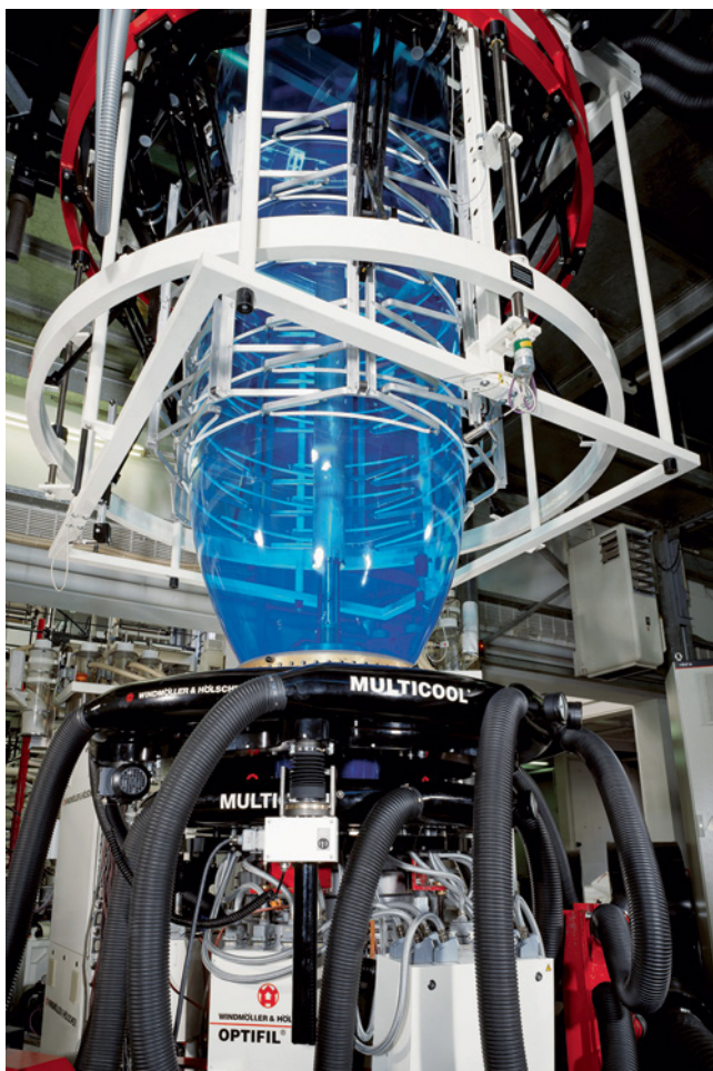
Figure 3 A blown film extrusion line ( Windmoeller & Hoelscher )
