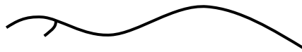
Figure 1.4 Schematic representation of an HDPE molecule showing high linearity with a small amount of short chain branching
