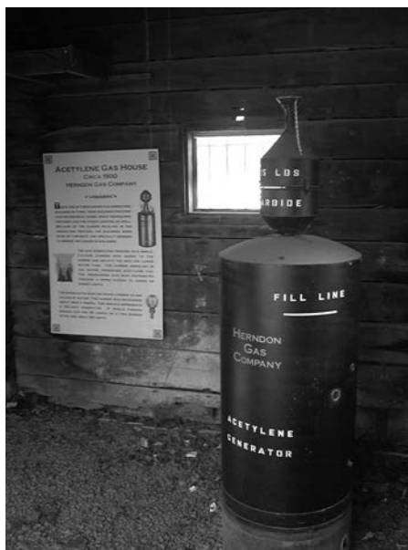
FIGURE 1.31 Acetylene gasmaking apparatus, preserved at Herndon, Virginia. (Authors' photograph).
