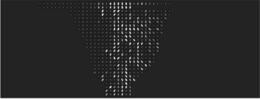
FIGURE 1.5: An illustration of the effect of grain structure on the path of ultrasonic waves through granular welds. Here we plot the magnitude of the dilatation.
