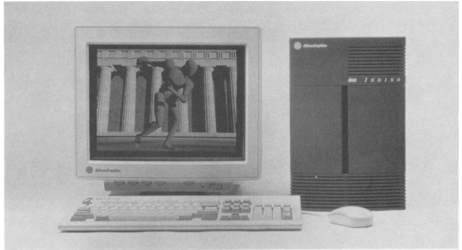
FIGURE 1.4 Photograph of a workstation. The cathode ray tube (CRT) screen is the primary output device, and the keyboard and mouse are the primary input devices. Photo courtesy of Silicon Graphics.
