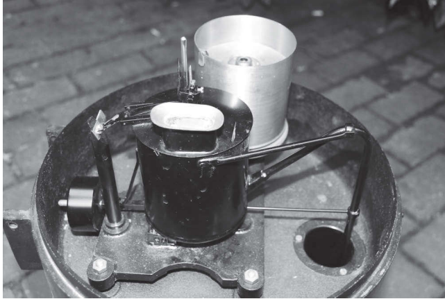
Fig. 3.4 The internal mechanism of a tilting-syphon rain gauge. The design is described in Met Office (1982) Observer's Handbook , 4th edition. Her Majesty's Stationery Office.
