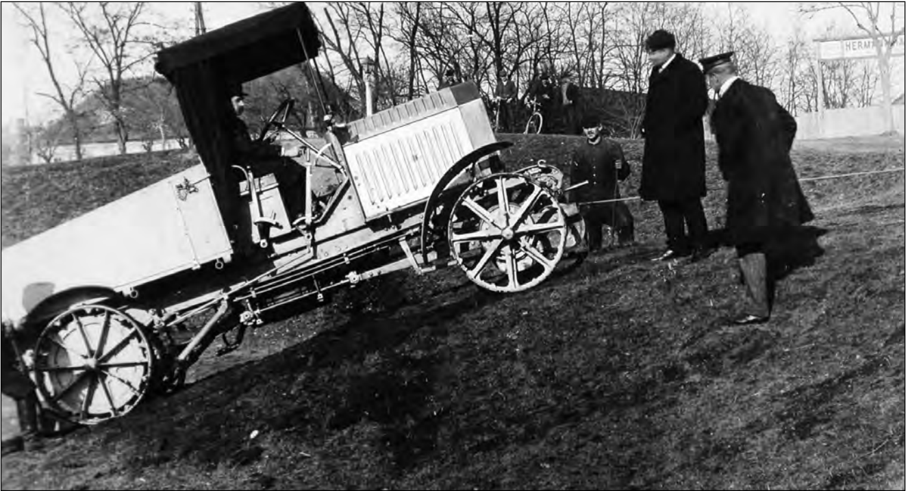
Elements of Paul Daimler's 1904 four-wheel-drive system contributed to Austro Daimler's first military tug, the M 06. It was one of the first 1906 projects of Porsche, testing its winch here with Eduard Fischer (right).
