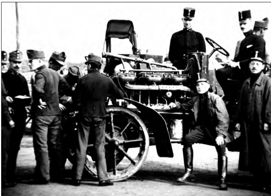
By 1910 troops in the field were getting to know the intricacies of the four-wheel-driven M 08 tug, including its impressive 13.9-litre six-cylinder engine developing 80hp.
