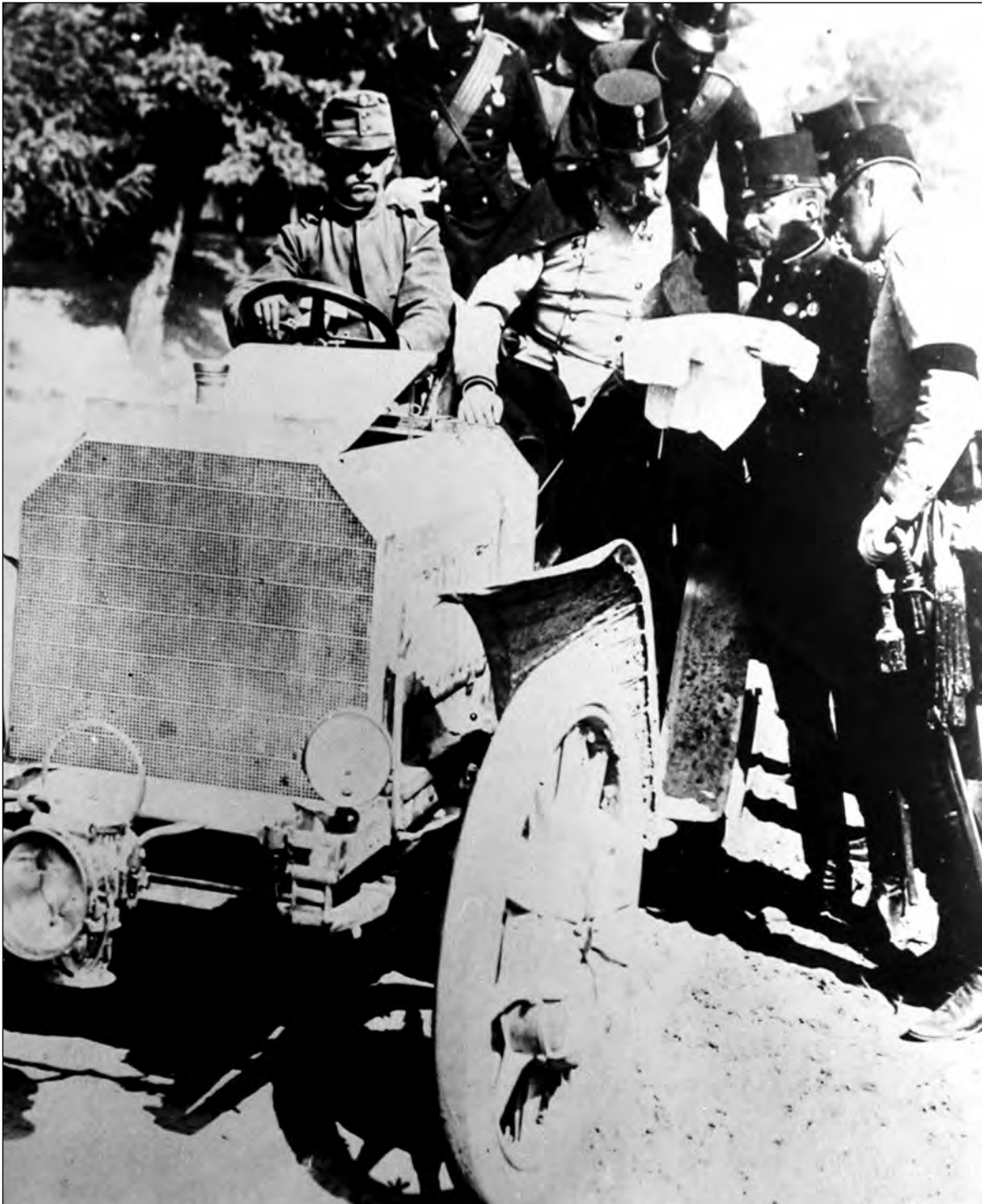
Reviewing maps of the manoeuvres in Austria-Hungary's Sárvár region, Crown Prince Franz Ferdinand was seated next to his driver Ferdinand Porsche in the latter's latest creation, which drove its front wheels through hub motors.
