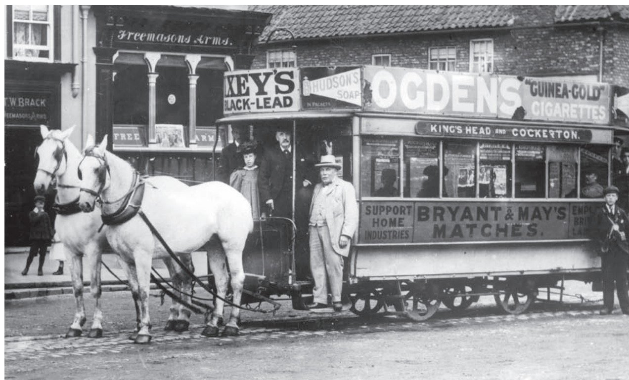
One of Stockton & Darlington Steam Tramway Co's 3ft 0in gauge horse trams stands in front of the Freemasons' Arms on Bondgate in Darlington. It is suggested that the elderly gentleman standing on the platform at the front dressed in white is from the company's then owners – Imperial Tramways. If that is the case, the image must date to between 1898, when Stockton & Darlington Steam Tramway Co was acquired by Imperial Tramways, and August 1903, when horse tram services ceased. Barry Cross Collection/Online Transport Archive
