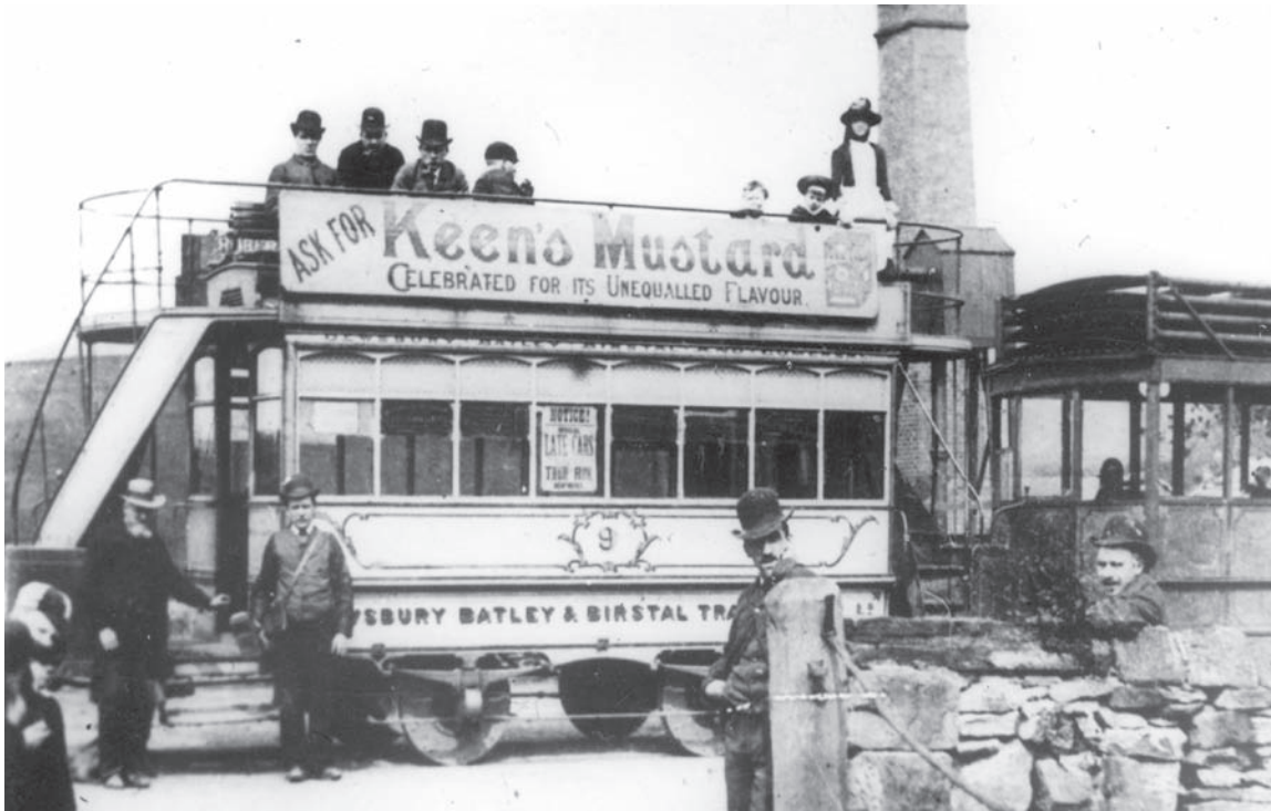
Steam trams were introduced by Dewsbury, Batley & Birstal Tramways Co on 10 April 1880. In all, eleven steam locomotives, all built by Merryweather, were operated over the 4 \frac{1}{4} route miles that the company leased. In 1880 one of the locomotives is pictured attached to ex-horse trailer No 9, one of five (Nos 6-10) built by Starbuck Car & Wagon Co between 1876 and 1880. Barry Cross Collection/Online Transport Archive
