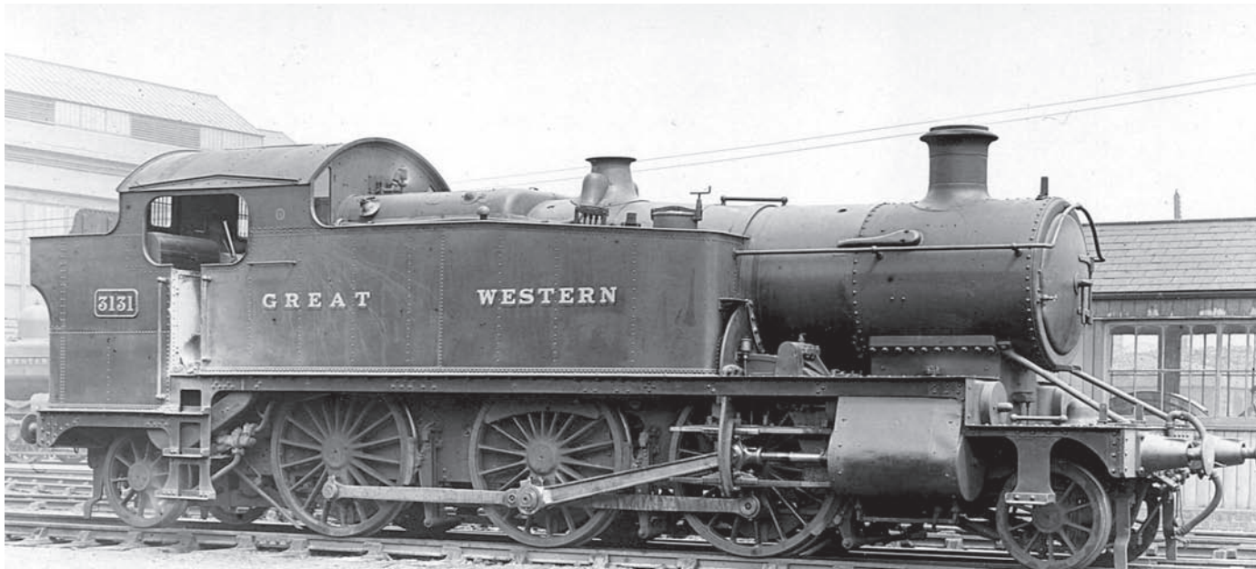
3156 of the 3150 class built in 1907 with the larger chimney, tall safety valve cover and enlarged bunker, c1920s. GW Trust Collection
