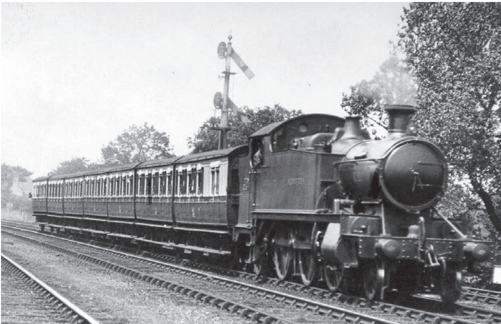
3100 class 3148 , built in March 1906, works a suburban train of Dean close-coupled six-wheel stock in the Birmingham area, in the immediate post-First World War period. As 5148 (renumbered in 1928) it was the last survivor of its class, outliving its sisters by over four years and not being withdrawn until December 1959. GW Trust Collection
