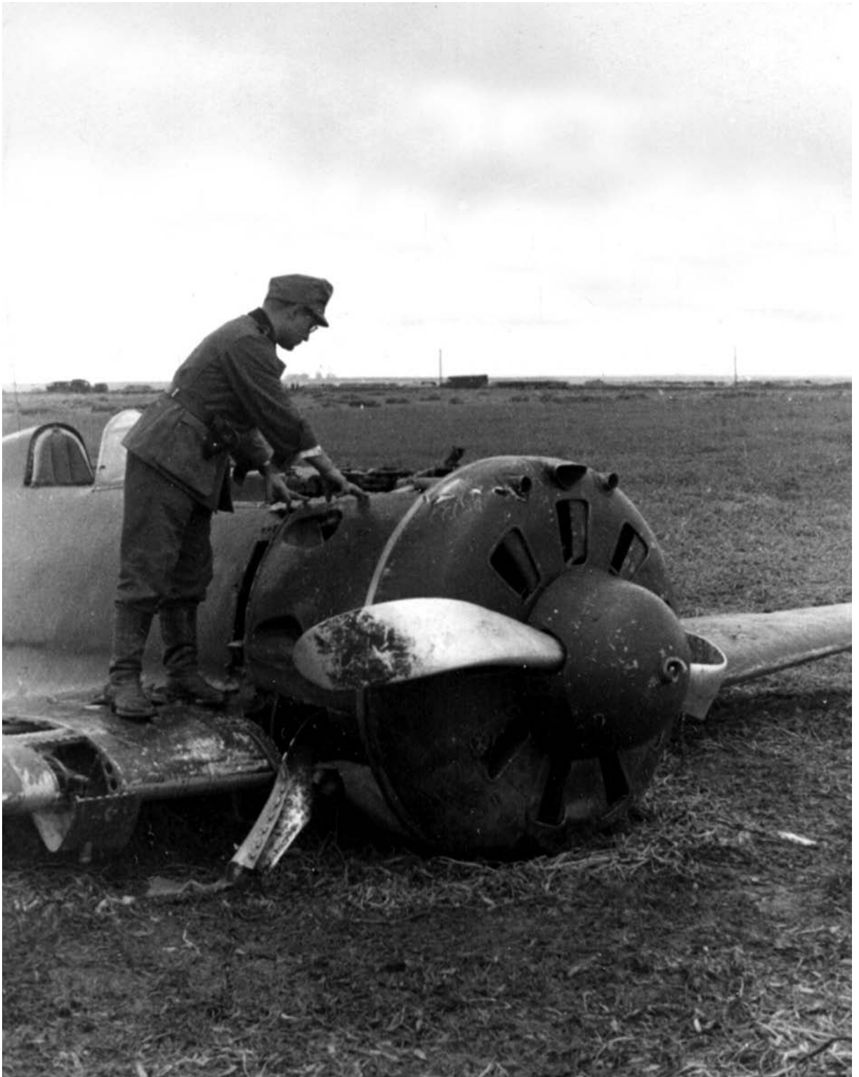
This Soviet wheels-up I-16 fighter; its propeller blades all bent out of shape, gets the once-over by a curious German soldier. It was possible for a pilot to survive such a heavy landing and live to fight another day.
