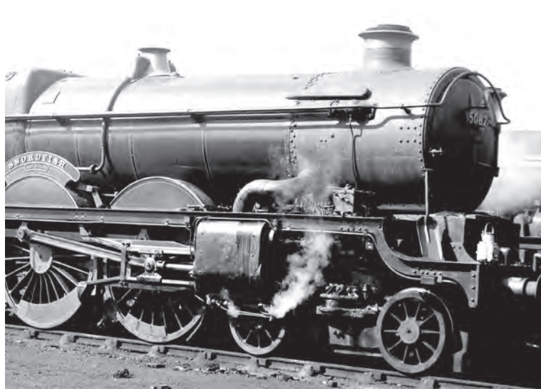
No 5082 SWORDFISH seen with 'modified' outside steam pipe, shorter chimney (introduced 1936) straight frames, box pattern inside cylinder casing (Nos 5013 onwards and BR straight frame rebuilds) BR pattern parallel barrel buffers and mechanical lubricator in the final forward position, circa 1961. David Anderson
