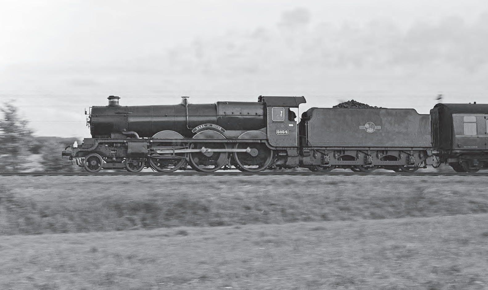
GWR 'Castle' class 4-6-0 No 5054 EARL OF DUCIE, this locomotive was renamed from LAMPHEY CASTLE. Seen at speed (recorded at 96MPH) passing Great Somerford with the Ian Allan 'Great Western High Speed Railtour', on 9th May 1964. Hugh Ballantyne/Rail Photoprints
