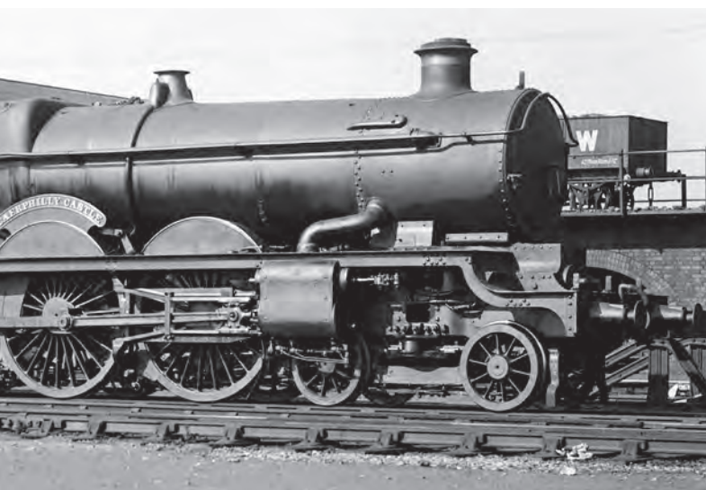
No 4073 CAERPHILLY CASTLE seen in original condition with 'tall type' chimney, 'straight' pattern steam pipes, 'joggled' frames, curved side pattern inside cylinder casing (Nos 4073–4092, ex 'Star' rebuilds and 4093–5012 straight framed engines) and GWR pattern taper barrel buffers, circa 1930. Rail Photoprints Collection
