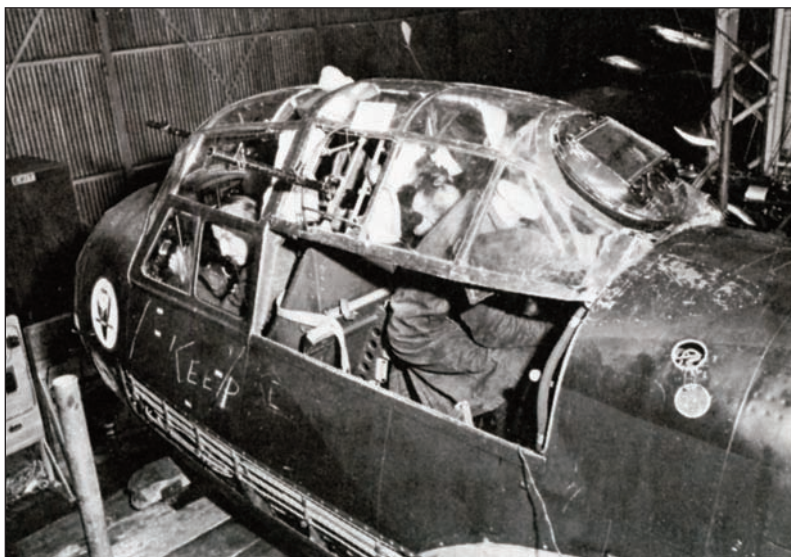
The cockpit section of Ju.88A-1 7A+FM under examination at the RAE. The aircraft made a wheels up landing at RAF Oakington on 19 September 1940. (John Hamlin Collection)
