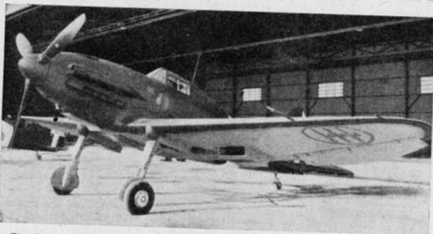
The Italian Caproni Reggiane 2001 single-seater fighter. It is powered by a Mercedes-Benz DB601N engine of 1,150 h.p. and has a maximum speed of 348 m.p.h. at 22,000 ft.
