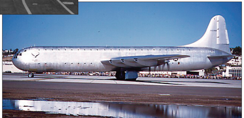
The Convair XC-99 - a civilian version - the Model 37 - was offered, but never built. It is seen here in the early colour scheme, without the nose-radar fitted and huge single wheel landing gear.
