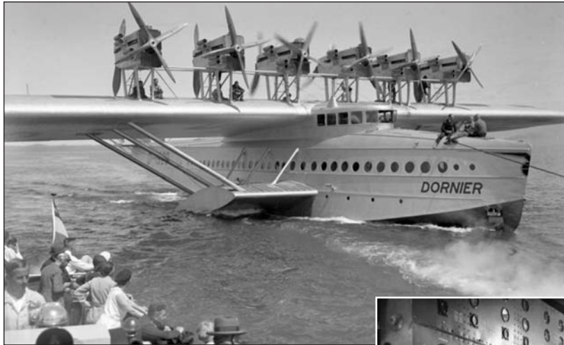
Above: The Dornier Do.X under tow, but with at least four of the twelve Curtiss Conqueror engines turning.
