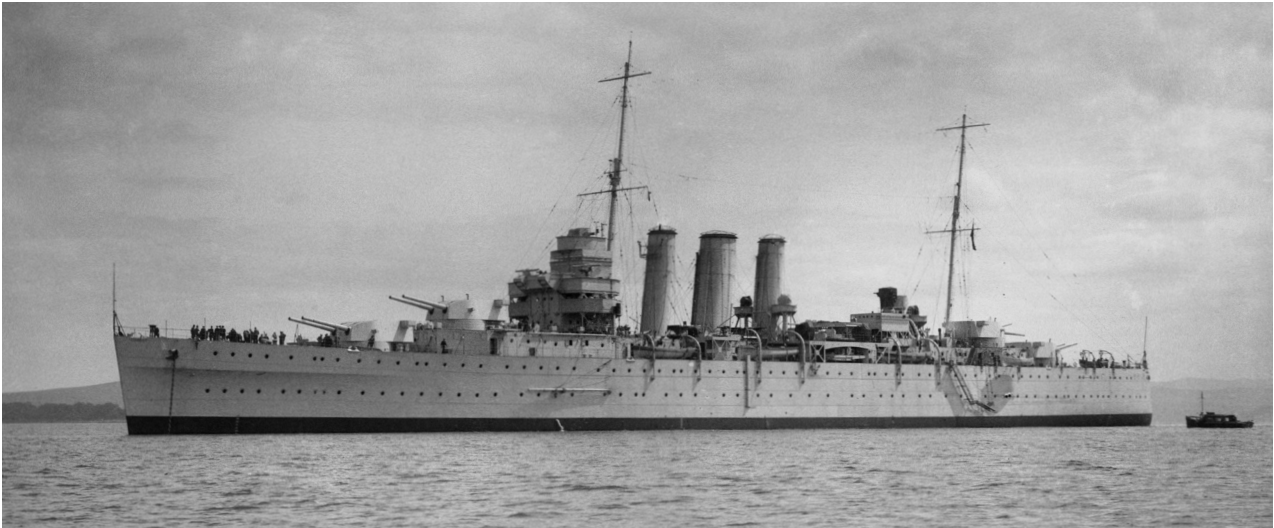
Shropshire as in 1929. Note the base for aircraft catapult but no catapult at this date (even the later ships completed without one). ( National Maritime Museum N8314 )
