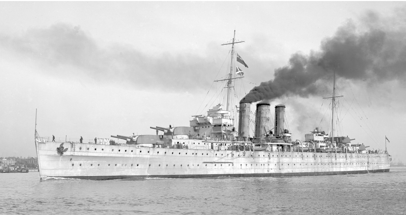
Dorsetshire in July 1930. The last pair were completed with a DCT and consequently the tall tower at the back of the bridge was omitted. (Wright & Logan Collection)
