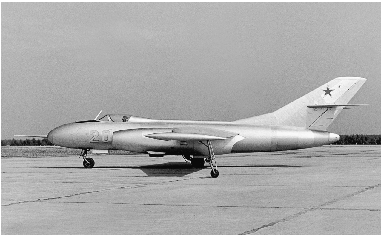
Side view of a production Yak-25RV ('20 Yellow'), showing to advantage the slim fuselage and the shape of the nosecone.
