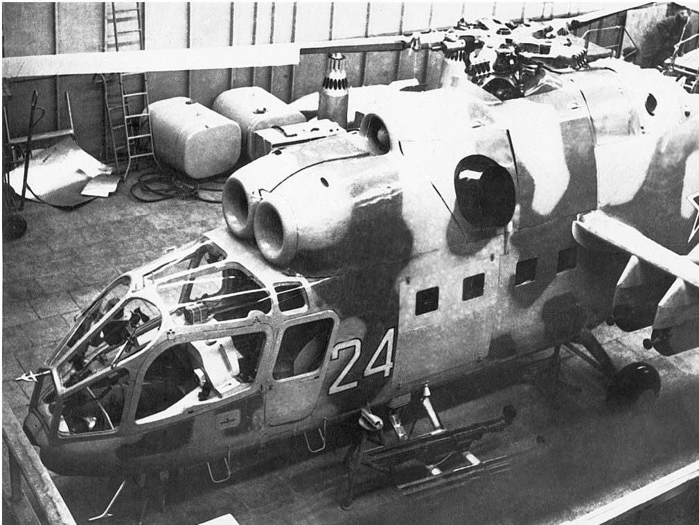
This aspect of the V-24 prototype (with markings added) during trials shows clearly the cantilever racks carrying the ATGM launch rails. Here, dummy bombs are suspended under the wings. Note the two portside cockpit doors.
