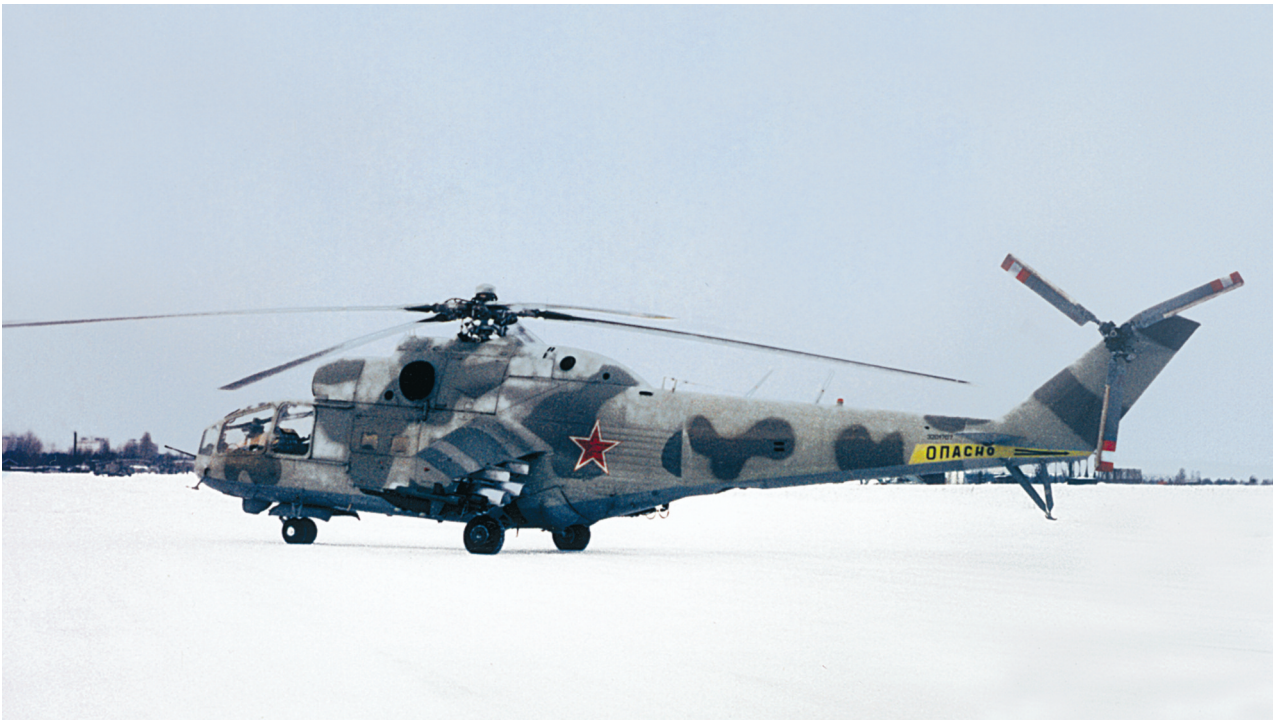
This page: '77 Red', the prototype of the Mi-24A, showing the anhedral wings with vertical endplates carrying the ATGM launch rails and the A-12,7 machine-gun in the nose. Note also the longer cockpit section.
