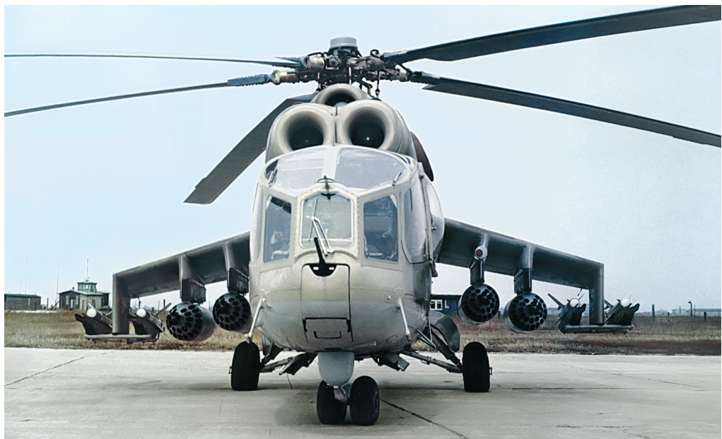
This page: '77 Red', the prototype of the Mi-24A, showing the anhedral wings with vertical endplates carrying the ATGM launch rails and the A-12,7 machine-gun in the nose. Note also the longer cockpit section.
