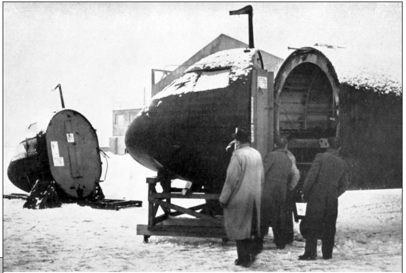
The windscreen rain clearance capabilities of the new design were tested 'in the real world' by putting a mock-up nose on the front of a Airspeed Horsa glider and flown from Hatfield during the bitter winter of 1946. (DH Hatfield)
