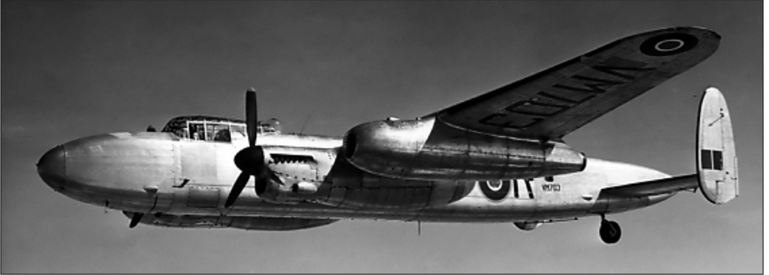
Once airborne the Lancaster flew on the outboard Ghosts alone. The tests were made by John Cunningham and Chris Beaumont, with a second Ghost Lancastrian VM729 added to speed the testing up. (DH Hatfield)
