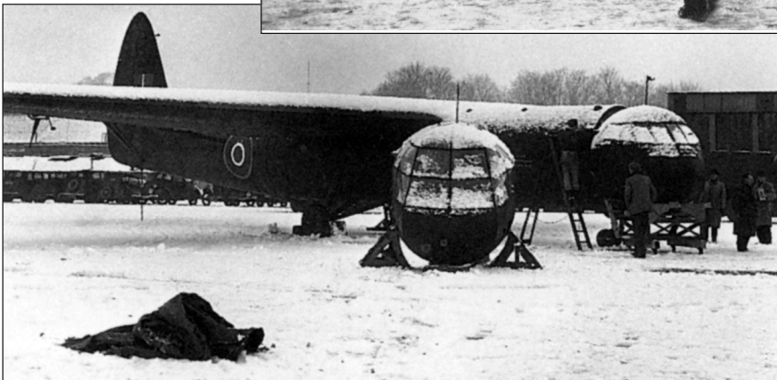
The windscreen rain clearance capabilities of the new design were tested 'in the real world' by putting a mock-up nose on the front of a Airspeed Horsa glider and flown from Hatfield during the bitter winter of 1946. (DH Hatfield)
