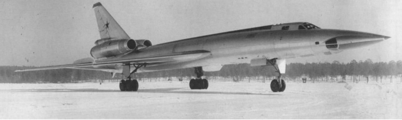
The first prototype of 'Aircraft 105', showing its resemblance to the eventual Tu-22, but differing in the nose area and more significantly, in the inward-retracting main undercarriage. OKB Tupolev
