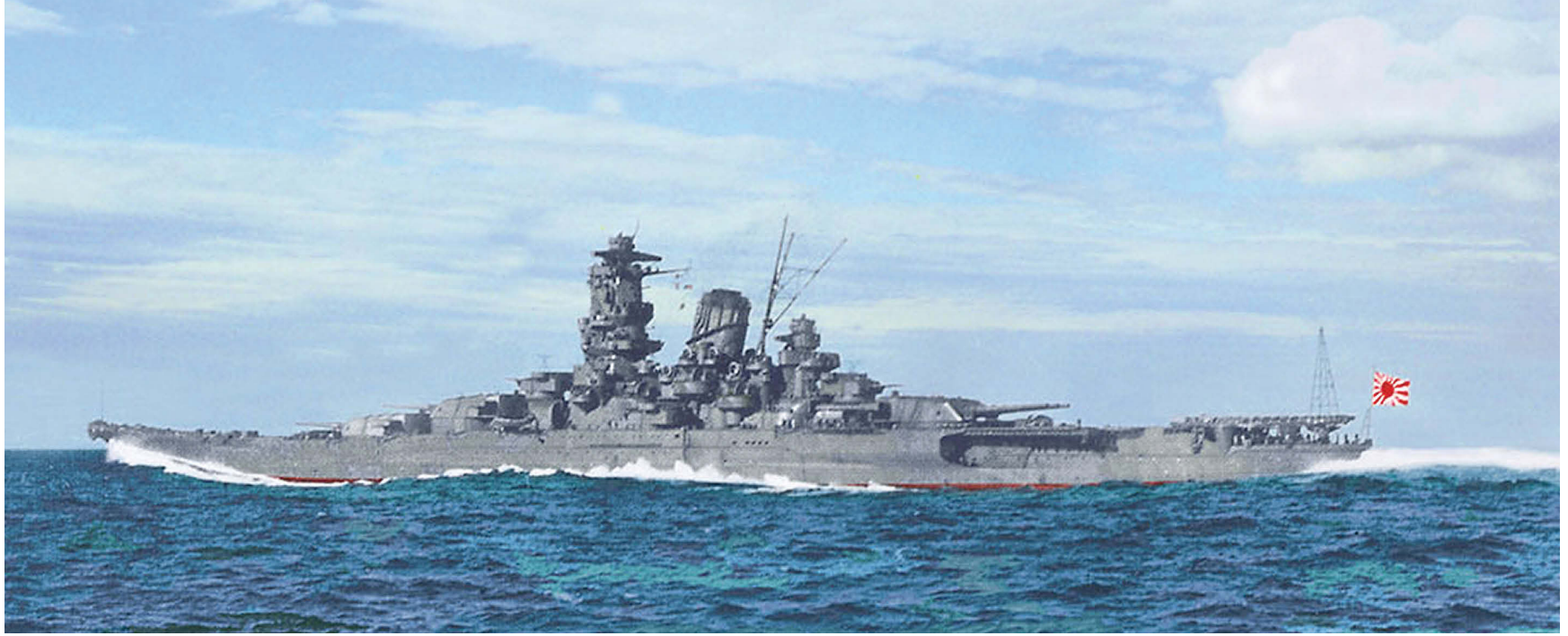
Quarter view of Yamato running builder's trials on 30 October 1941. The boat stowage hangar, catapult and lattice antenna mast on the crane platform are clearly visible.
