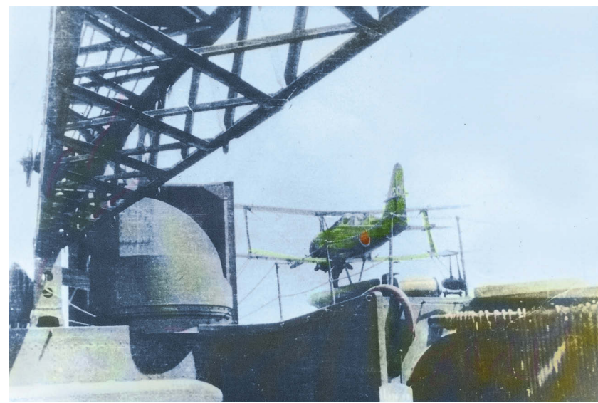
A Mitsubishi F1M2 floatplane aboard Musashi seen from under the aircraft crane, January 1944. The new type MG control tower can be seen on the left, and in the right foreground the sisal rope curtain that closed off the boat stowage.
