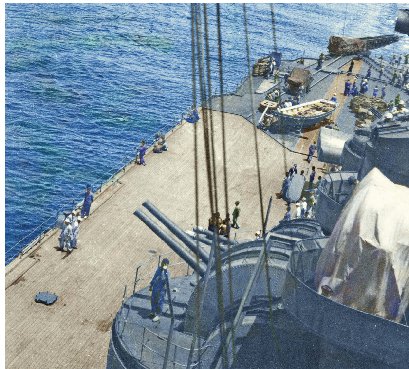
The division between the wooden deck and the steel aircraft deck is clearly visible in this view of Musashi from July 1942. Note the twin 12.7cm HA gun mount in the foreground and the canvas-covered 150cm searchlight.
