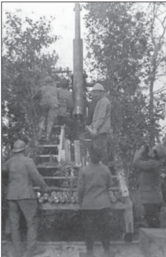
French soldiers adapt their versatile 75 mm field gun to anti-aircraft use against a German bomber. Rings of such guns surrounded balloon nests, creating a cone of fire around an endangered gasbag as it was winched down (Jon Guttman)
