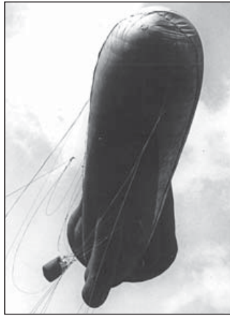
This Caquot type balloon caught in a heavy gale shows the improved stability that its three fins afforded compared to the Drachen's single ventral stabiliser. In consequence, the Caquot design began eclipsing the earlier type in armies on both sides of the lines from 1916 onwards (IWM Q27265)
