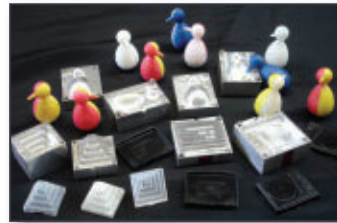
Stanavich is also using his PCNC 1100 to machine the permanent molds for toys he uses as unique calling cards for the shop.
